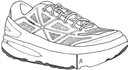
Fig. 5.9. The Hoka One One Mafate can have as much as 1½ inches (37 mm) of midsole cushioning (A).
