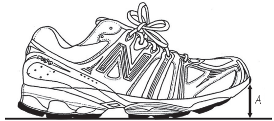
Fig. 5.5. The typical running shoe is manufactured with a toe spring (A), which allows the foot to move in a more natural manner and reduces strain on the Achilles tendon and plantar fascia.
